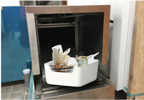
The conveyor stops when the basket arrives at the end, where the staff can remove the basket and place it at the washing area for the conveyor to continue moving.
